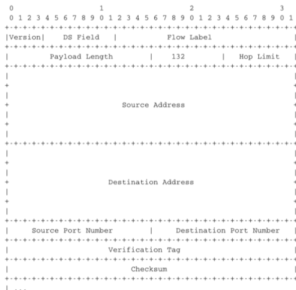
Figure 3.48: An IPv6 packet containing an SCTP segment
