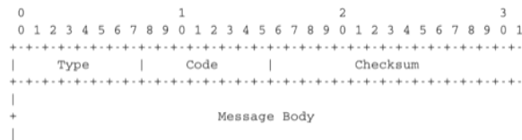
Figure 3.54: ICMP version 6 packet format
