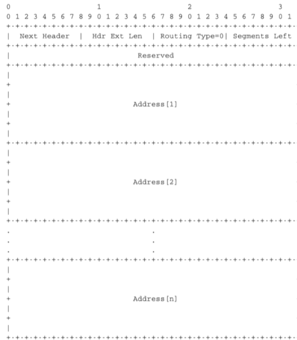
Figure 3.53: The Type 0 routing header (RFC 2460)
