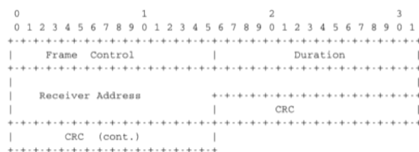
Figure 6.35: IEEE 802.11 ACK and CTS frames
