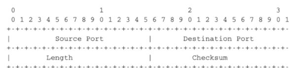
Figure 4.34: UDP Header Format
